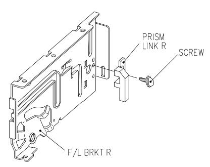
Fig.3-3 DISASSEMBLY OF THE F/L BRKT R
